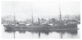
40 foot beam. She had three masts and was barquentine rigged as auxiliary power for the main steam propulsion. The ship struck an uncharted rock now known as Quetta Rock. The 133 survivors of the
